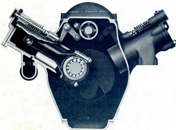
End View of V Engine, Showing Connecting Rod, Piston and Valve Action
