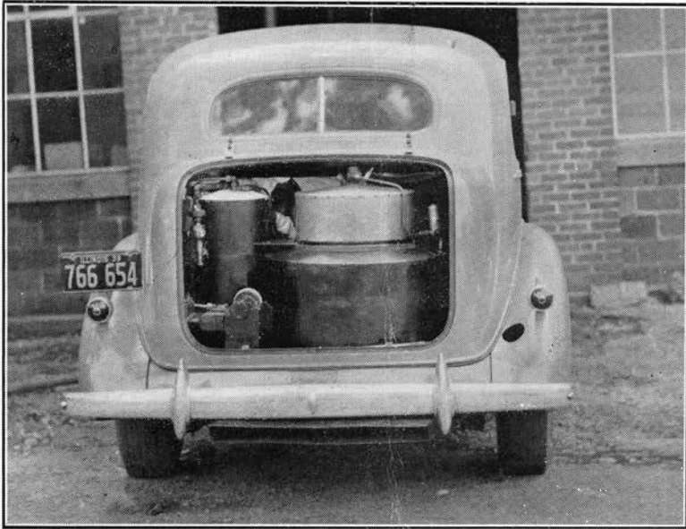
Fig 3.—REAR VIEW OF THE LESLIE CAR, SHOWING THE NEW BOILER.
